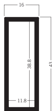
Z 100 Beam extrusion 43 mm 3.14 kg | 5000 mm
