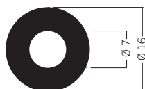
M 1460 Round extrusion 16 mm 2.57 kg | 6000 mm
